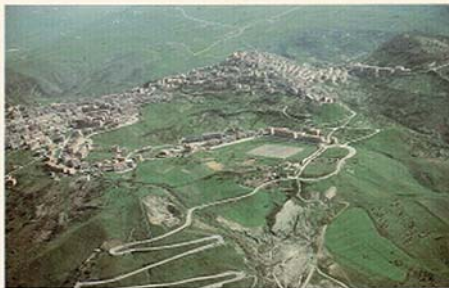
Fig. 75 - Calitri Aerial view of upper part of landslide mobilized by the 1980 earthquake.
